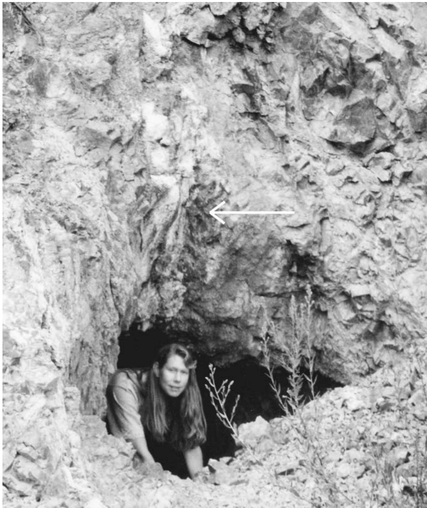
Figure 1.3. Amanus Mountain Mine Entrance near Kisecek Showing Vertical Vein of Arsenopyrite/Chalcopyrite with Heidi Ekstrom as Scale. Photograph by K. Aslihan Yener
