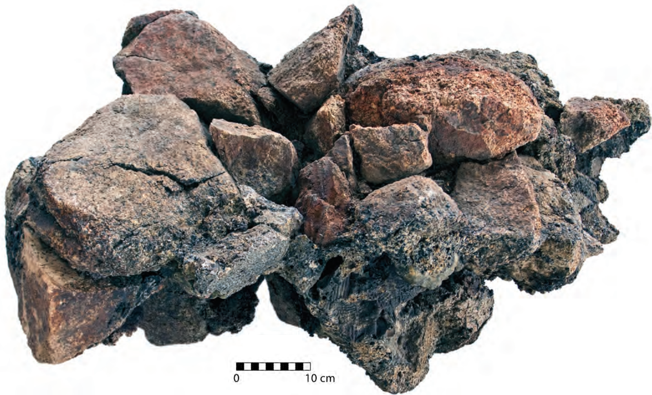
| (a) Granite, partially vitrified with some mud and wood impressions
