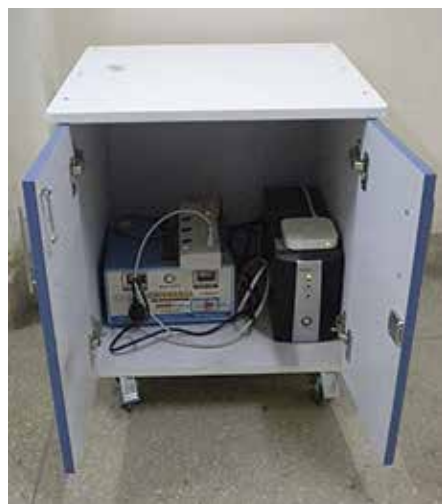
Figure 3. Router extender in a cabinet on wheels – our two “rolling routers” enable the Kabul team to extend our wireless network to reach every gallery and storeroom in the National Museum so that we can carry out the data entry for the museum inventory
