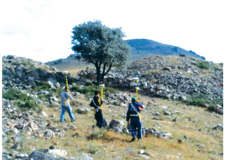
**GPS survey in action with three roving receivers**
