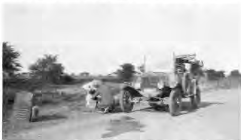
FIG. 13.—Fitting new bearings to the Ford en route to Minyeh
