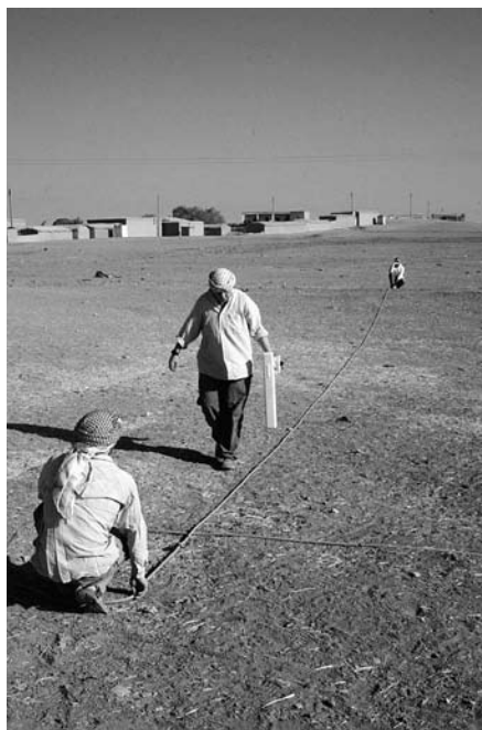
Fig. 1. Collecting data with the magnetometer at Hamoukar’s lower town
