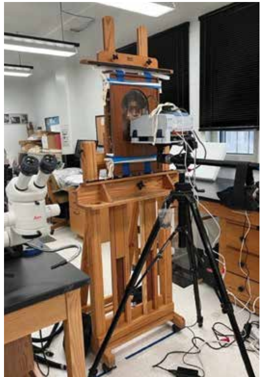
Figure 9. Female funerary portrait undergoing Fourier-transform infrared spectroscopy to aid in identifying materials and pigments.
