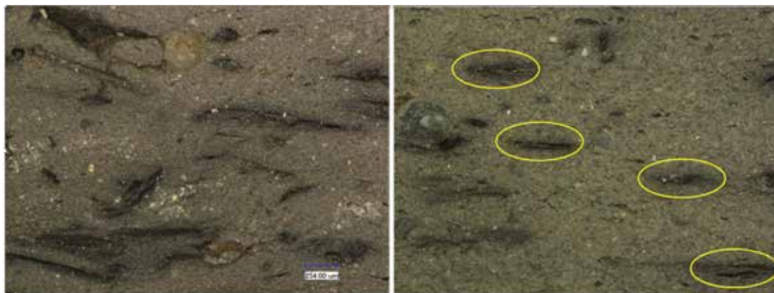
Figure 7. Microphotographs (100×) of high-arsenic sherds taken under incident light. Note the platey rock fragments circled in the image on the right.
