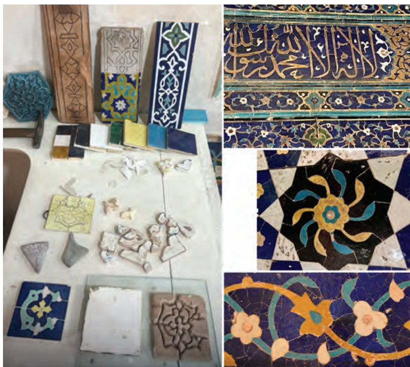
Figure 4. Stages in the production of glazed cut-tile mosaics (left); cut-tile mosaic technique used for calligraphic (top right), geometric (center right), and floral (bottom right) designs.
