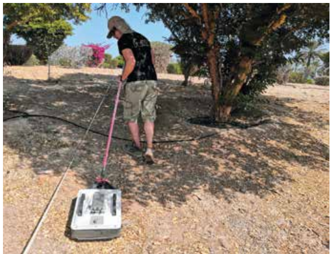
Figure 3. Ground-penetrating radar survey in process.
