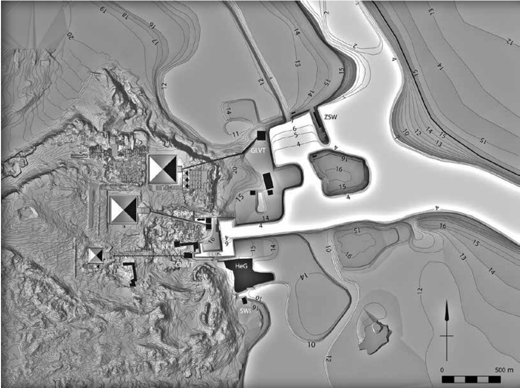
Figure 22. Reconstruction of Fourth Dynasty water transport infrastructure at Giza, with contour values in meters above sea level; white indicates low water level at 7 m asl; ZSW = Zaghloul Street Wall; HeG = Heit el-Ghurab site (map: Rebekah Miracle from AERA GIS, based on design by Mark Lehner)
