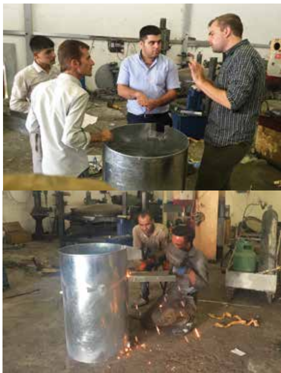
Figure 12a-b. Lucas Proctor consulting with Erbil metal-workers on design of the flotation machine (top) and the final assembly of the flotation machine (bottom)
