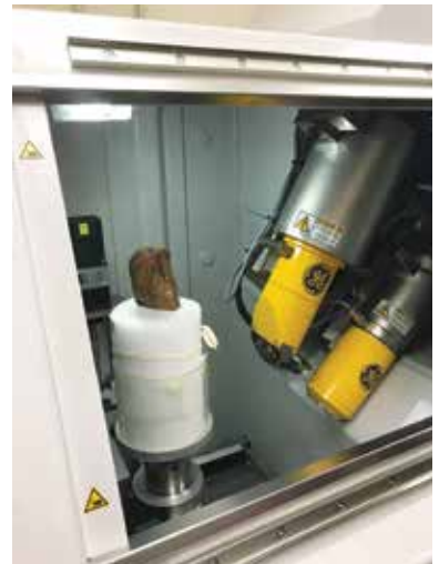
Figure 4a-b. E119, bird mummy, in its custom made mount (top) and inside the PaleoCT high resolution scanner at Biological Sciences Division (bottom)
