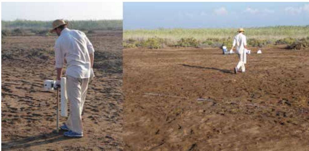
Figure 4. Gradiometer calibration and ongoing geomagnetic survey along the grid axes
