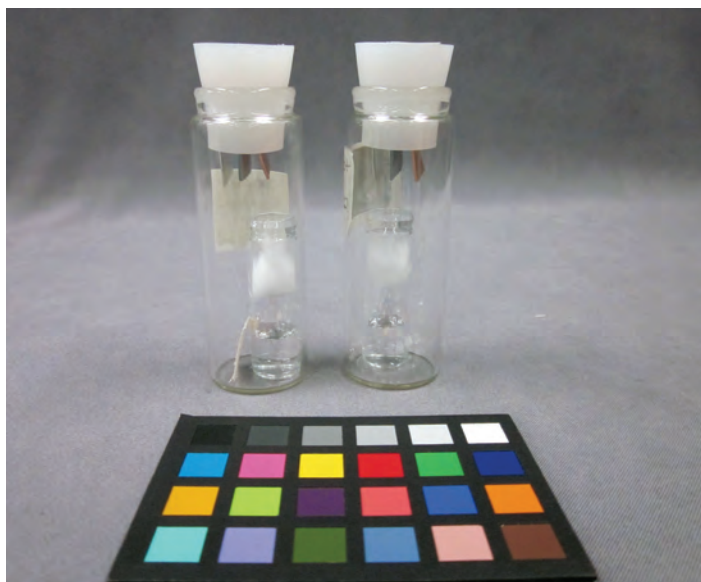
Above: Oddy test of fabric (left) and control (right). Right: Coupons placed in the display cases (1 and 2) compared to a set of control coupons (3).
