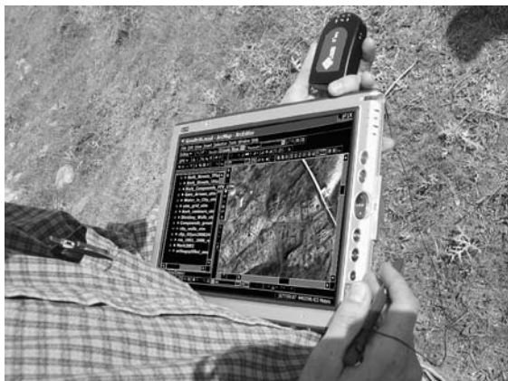
Figure 5. Ground-truthing with the GPS-enabled tablet PC. The GPS allows users to see themselves in real time within the imagery (a small gray circle in the center) and where they are relative to buried structures or streets. The tablet computer also allows users to draw directly on the screen to produce plans of the urban architecture in the field. This same system also works in a vehicle, just like an onboard car navigation system, to allow project members to drive along the network of buried city streets
