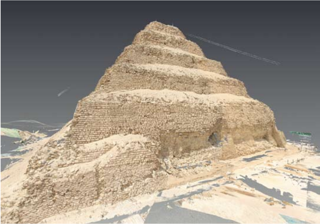
Figure 15. Point cloud model of the Djoser Step Pyramid, eastern side. Looking like an infrared photograph or negative image, the model is assembled from five hundred million points located precisely in space and arresting the pyramid in time: late May–early June 2008
