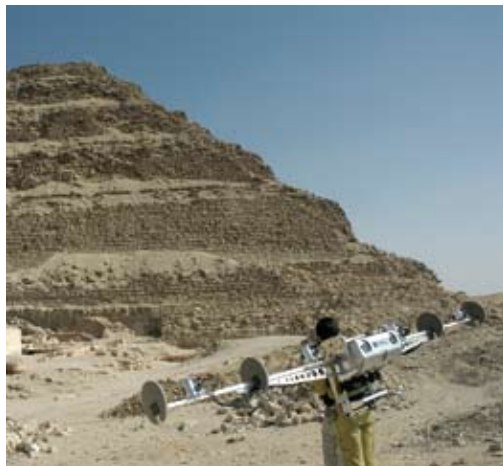
Figure 14. A climber about to ascend with the Zoser Scanner mounted on his back. Each wing of the device carries two miniature laser scanners and two miniature macro cameras. The scanner also sports a cooling system, a gyroscope, and a prism for tracking location
