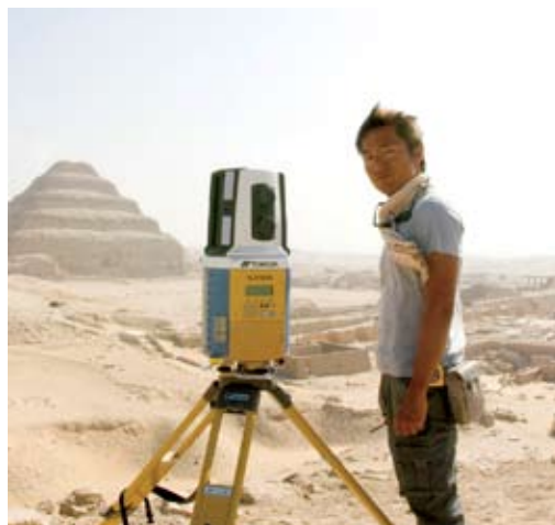
Figure 12. Yukinori Kawae, who organized the SLSS for AERA, at one of two Topcon GLS-1000 laser scanners that the team used for the preliminary overall survey of the Djoser Step Pyramid
