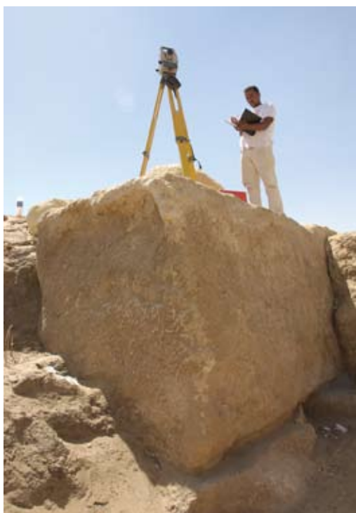
Figure 8. Surveyor Azab Ahmed Hassan stands with his total station on a massive core block of the MVT, which we exposed when we cleared a large hole at the northeast corner of the MVT. Each day when he set up on survey point GIII.1 of our Giza Plateau Survey grid, he rose higher and higher as we cleared deeper and deeper
