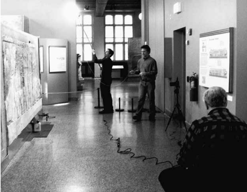
Figure 1. Highlight-RTI imaging of Khorsabad relief in the Oriental Institute Museum: Clinton Moyer (left) and Miller Prosser move the light; Kenneth Zuckerman (back to camera) controls camera and light; reflective red ball at base of relief registers light position
