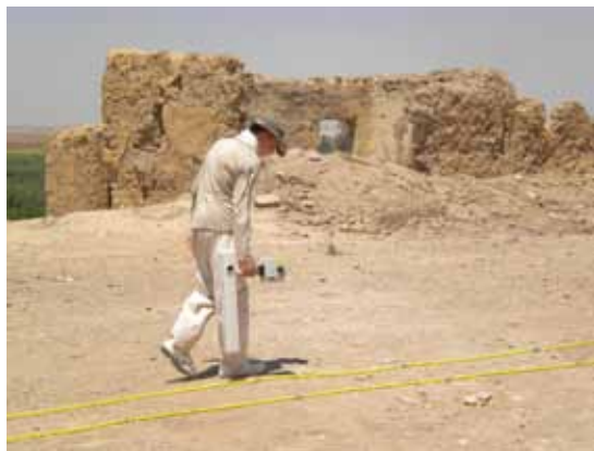
Figure 14. Andrew Creekmore conducting the geophysical (magnetometric) survey of Tell Zeidan, using a hand-held gradiometer
