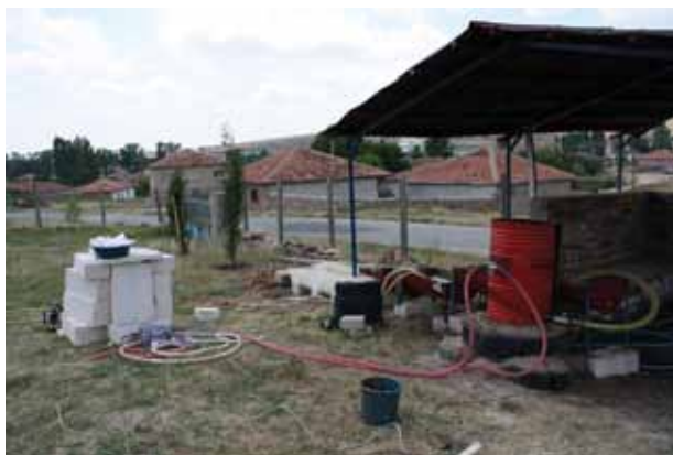
Figure 8. The new flotation machine all set up. This machine incorporates multiple water settling tanks to minimize overall water usage
