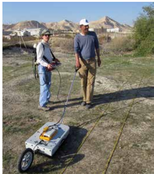
Figure 5. Andy and Jehad with ground-penetrating radar
