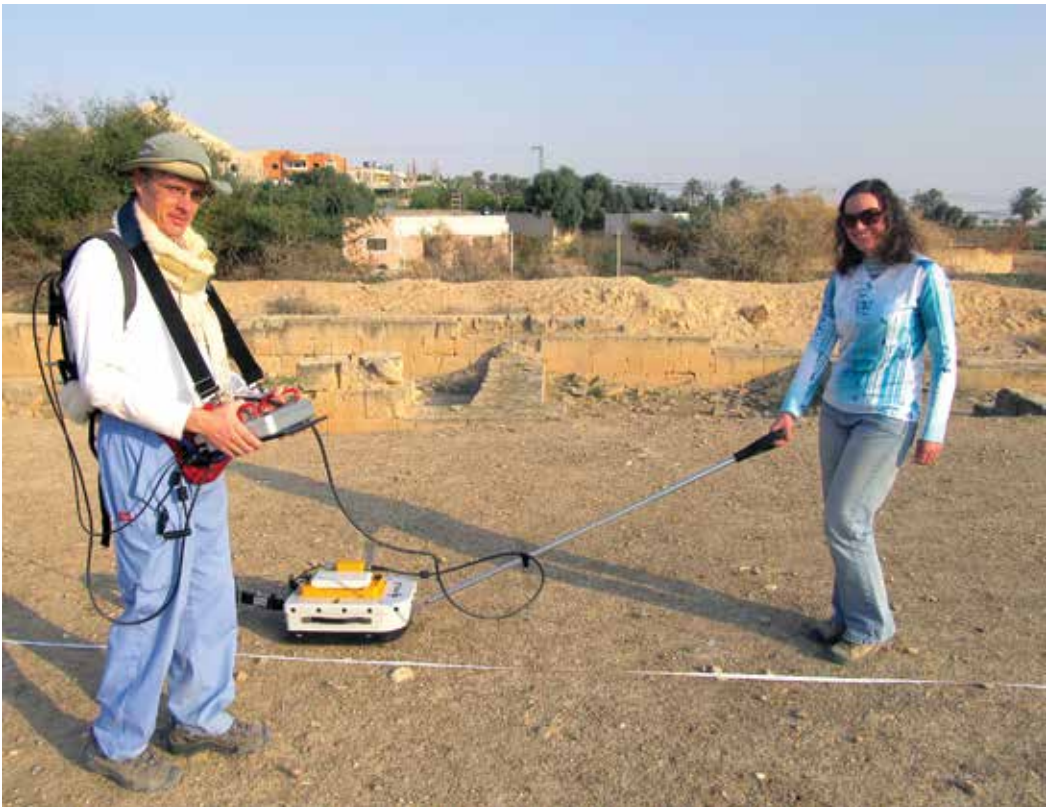
Figure 1. Andy and Ellie using the ground-penetrating radar in remote survey, area 1 (RS 1)
