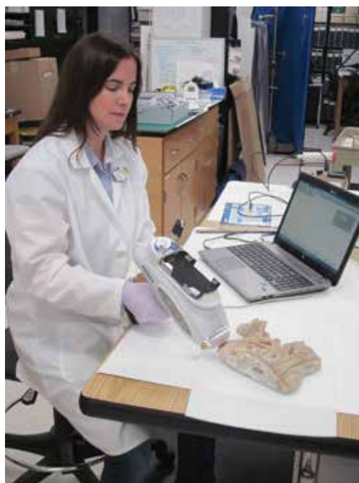
Figure 2. Associate conservator Alison Whyte analyzing pigment on a stone object using the Bruker Tracer III-SD pXRF device in the Conservation laboratory
