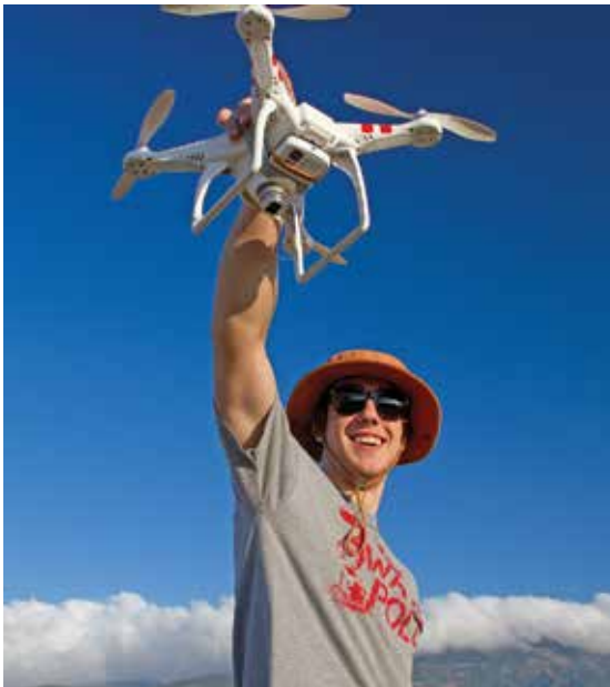
Figure 7. Expedition team member Robert Schloen with the remote-controlled quadcopter ("drone") to which a small camera was attached to take aerial photographs used in mapping the excavation areas with the aid of photogrammetry software
